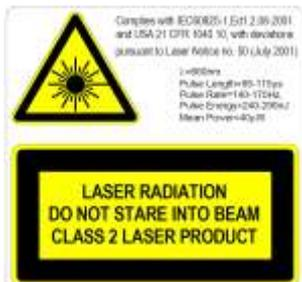
CSN950MH is fitted with Class2, visible (red) laser diode at wavelength 660nm. The laser warning label on the outside of the unit contains details about laser emission.
