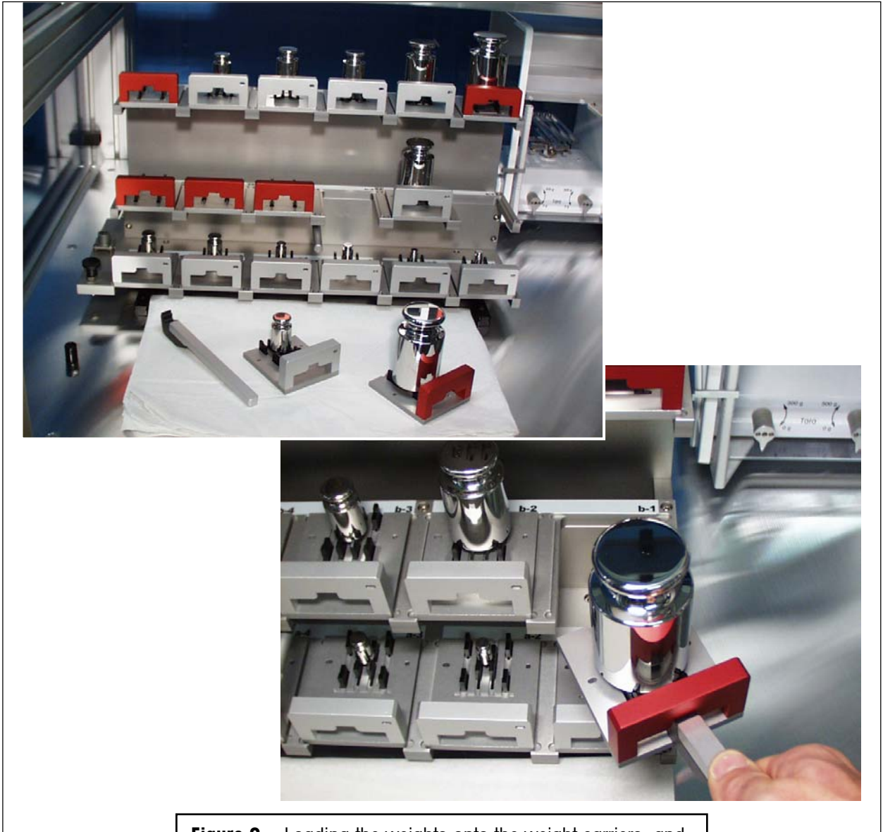
Figure 2 Loading the weights onto the weight carriers, and the weight carriers onto the weight magazine
