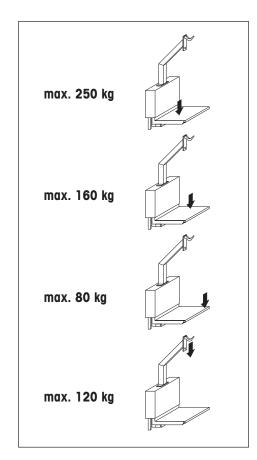
The wall scale has an extremely rugged construction and hence suffers no damage if the maximum weighing load of 150 kg is exceeded on the odd occasion.
