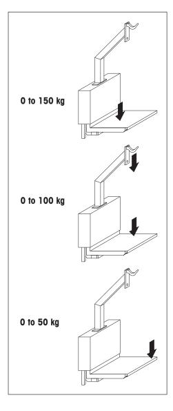
In the case of a **central** load, the weighing range covers the entire range from zero to the maximum capacity of the hinged plate.
