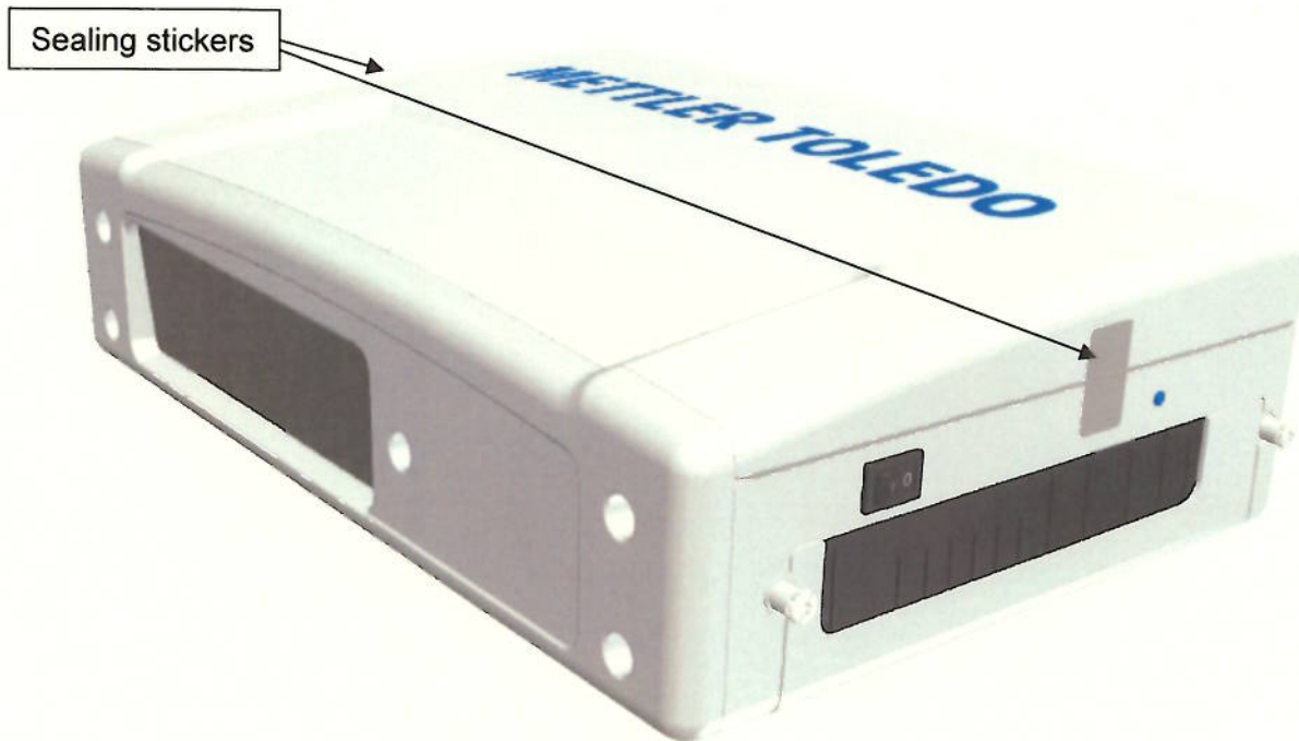
Figure 2 - Sealing of CSN950 top cover. Two sealing stickers shall be placed on opposite sides of the instrument. Each sticker shall overlap the housing and the top cover as shown in this picture.
