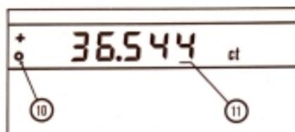
If an object is placed on the weighing pan, the last digit (11) is blanked out briefly. The weight should be read only when the last digit (11) reappears and the stability detector lamp (10) is off.
