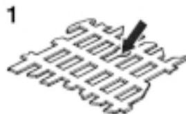
Check if the protective screen of your LP16-M dryer has a keyhole-like perforation according to **Fig. 1**.
