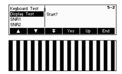
In order to check if the screen is functioning properly, press **«Yes»** and...
