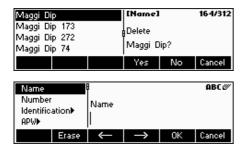
Press «**Delete**» to remove the current article from the database. You will be asked to confirm deletion of an article.
