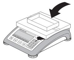
Place the **empty** weighing container or packaging on the scale and then press the  $\rightarrow T \leftarrow$  key briefly, or press the  $\rightarrow T \leftarrow$  softkey if a **known tare** weight has already been established.
