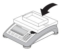
Place **empty** container on the scale and tare with the  $\prec \rightarrow T \leftarrow >$  key.
