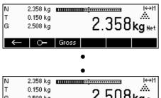
Press the «Gross» key. This function causes the gross weight to be displayed (the "G" symbol appears and replaces the "Net" symbol).
