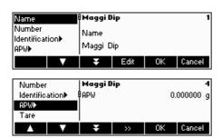
Press **«Define»** to modify the selected article. Select the desired parameter by using the **«II»**, **«II»**, or **«II»** softkeys, then press **«Edit»** to modify the selected parameter.
