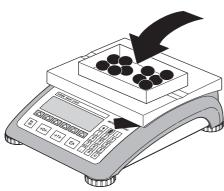
$\dots$  place 10 pieces of materials to be weighed to determine the reference weight.
