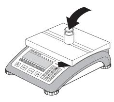
After choosing the calibration weight, place the weight on the weighing pan and then press the **«OK»** key.
