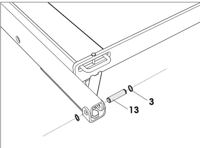
**EN** Place frame with weighing platform on the mounting plates and attach with the pin (13). Attach circlips (3).
