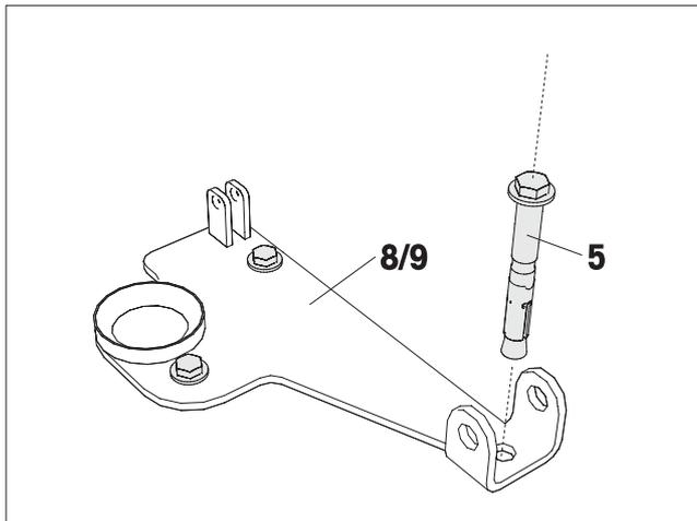
**EN** Attach first mounting plate (8/9) to the floor with 3 heavy-duty plugs (5).
