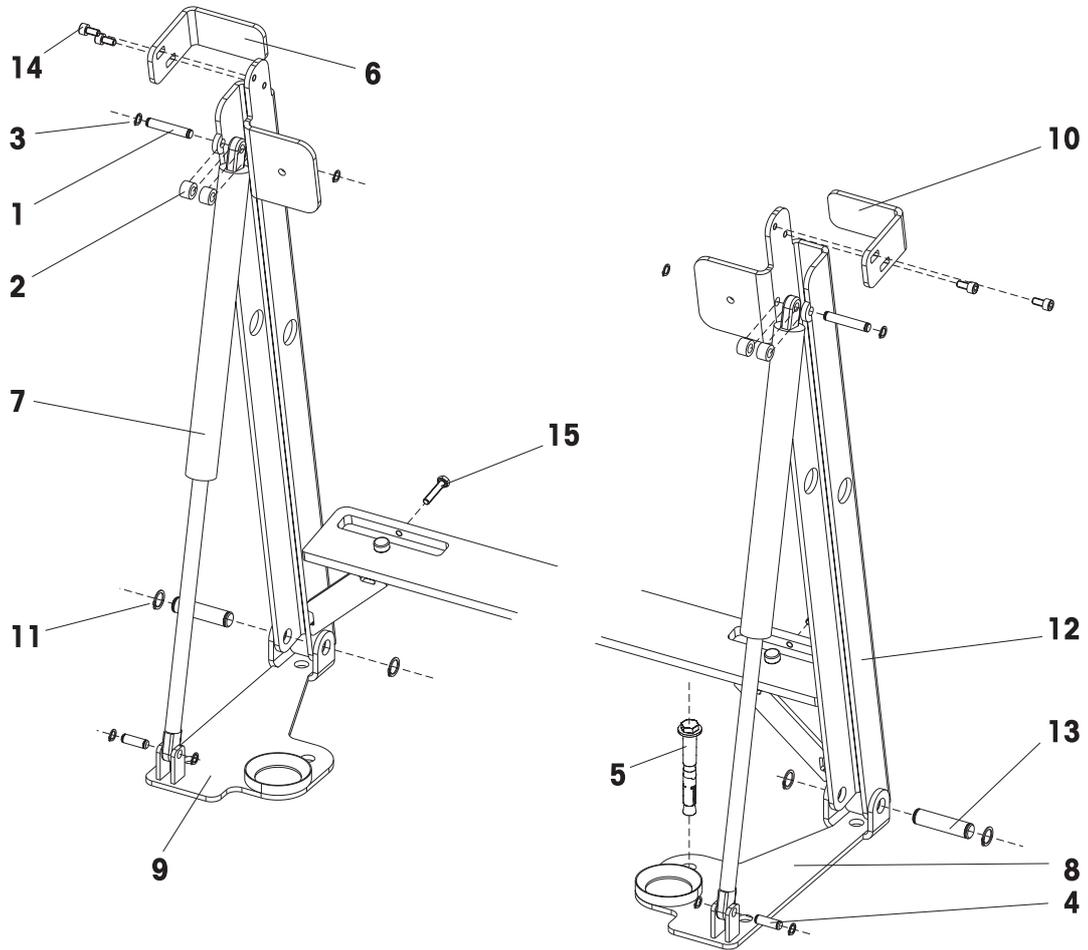
**EN** Installing lifting system**DE** Hebevorrichtung installieren**FR** Installer le dispositif de levage
