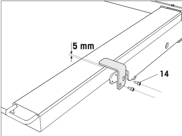
**EN** Attach bracket at the frame of the lifting system with M6x12 screws (14). When doing so, ensure that the space between the weighing platform and bracket is approx. 5 mm.
