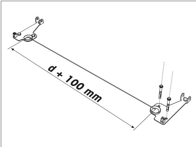
**EN** Ensure that the spacing of the levelling feet in the mounting plates corresponds to the passage width of the scale  $d + 100 \text{ mm}$ .
