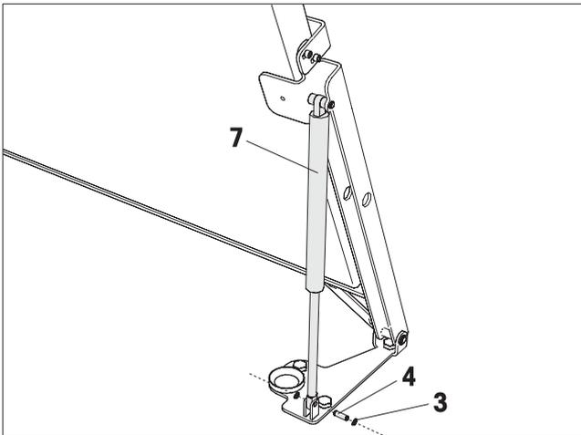
**EN** Fold up weighing platform and secure it. Connect gas compression springs (7) at the mounting plates with the shafts (4). Attach circlips (3).
