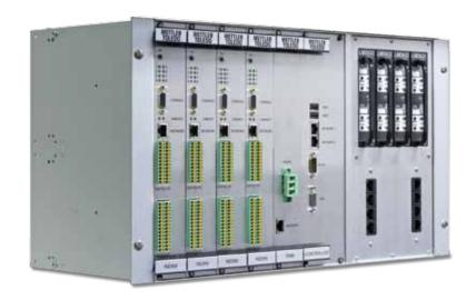
A high-speed data interface automatically records vehicle data and transmits it from WIM sites to a remote office.
