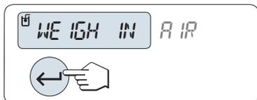
The balance prompts you to weigh the sinker in air "WEIGH IN AIR".
