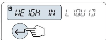
The balance prompts you to weigh the solid in the auxiliary liquid **"WEIGH IN LIQUID"**.
