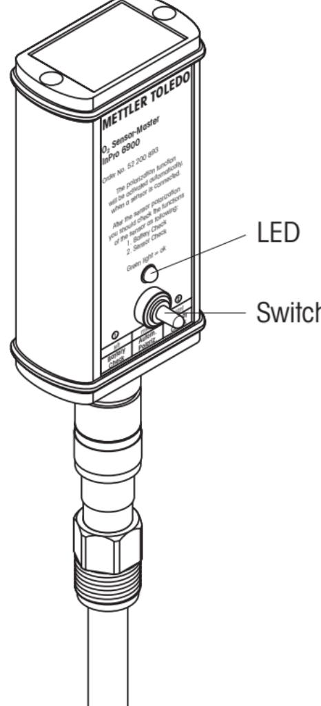
As soon as the sensor is connected to the O<sub>2</sub> sensor master, the polarization function is automatically activated. Please note: if the sensor was disconnected from the transmitter for longer than 5 minutes, the sensor must be polarized first (polarizing time see "Section 5.1") to get representative test results.
