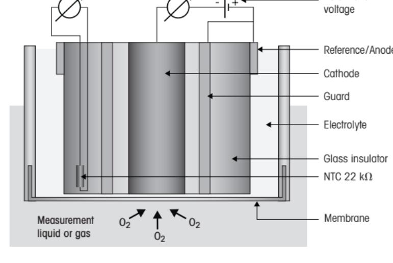
In all sensors the function of the cathode is identical.
