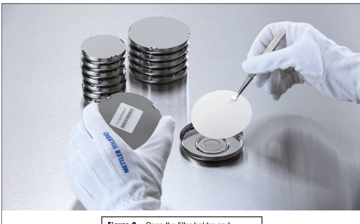
Figure 6 Open the filter holder and put the filter into the filter holder
