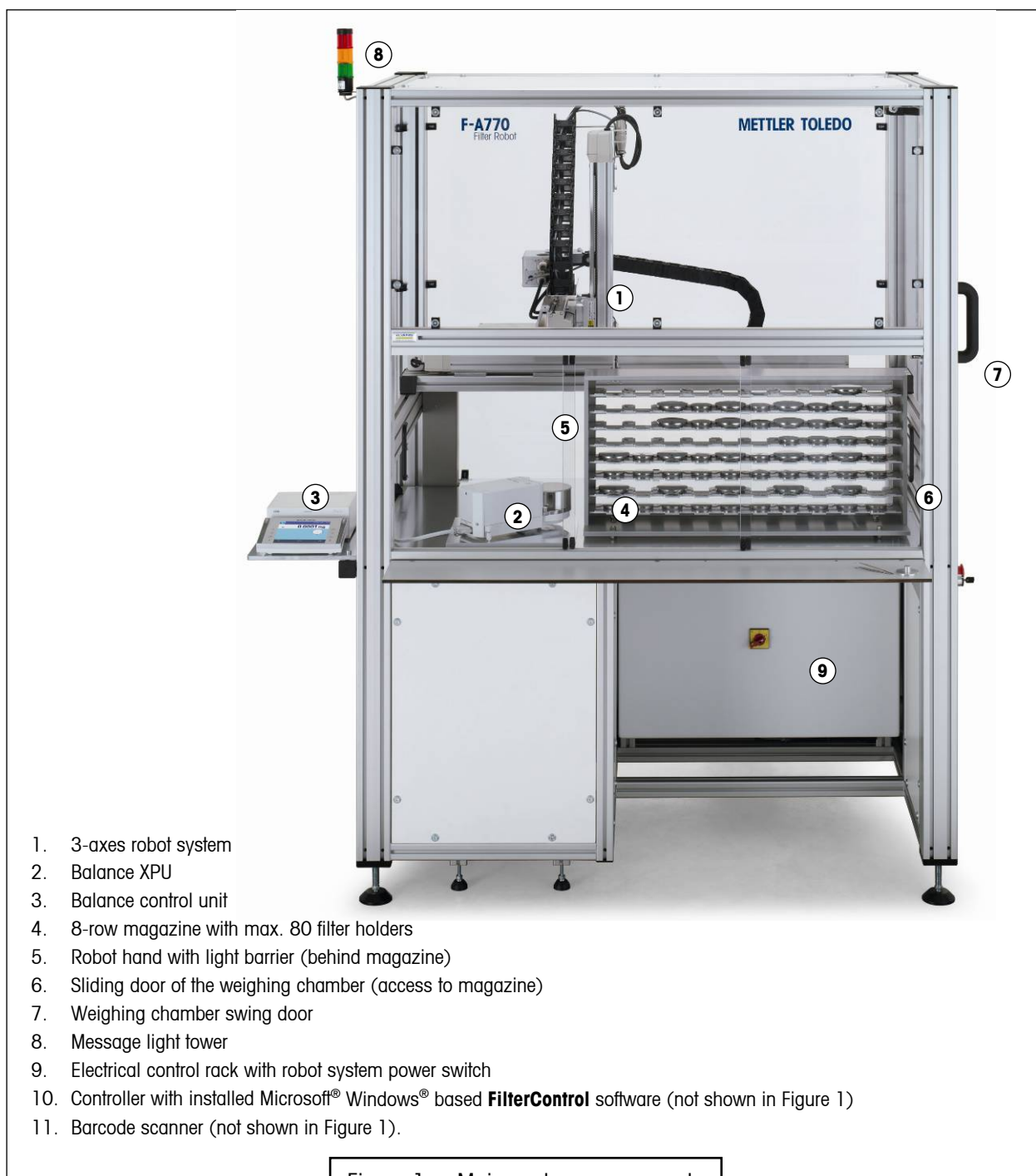
Figure 1 Main system components
