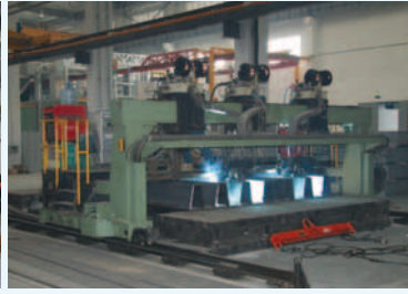
VTS202/302 are machine welded to obtain the best weld quality and long life
