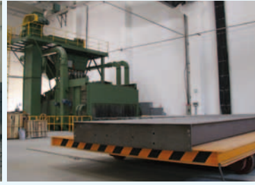
The steel in each VTS202/302 is shot blasted to create a fantastic painting surface
