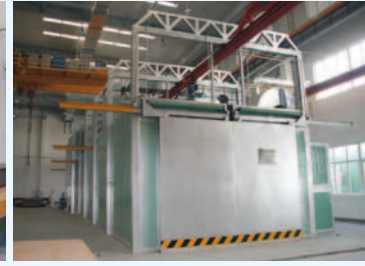
Each VTS202/302 is acrylic polyurethane painted and temperature cured to eliminate corrosion
