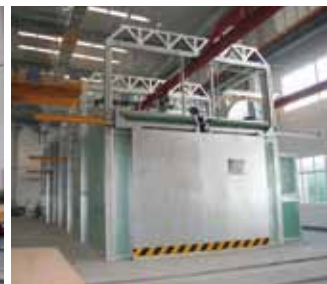
The VTC205 is epoxy painted and temperature cured eliminate corrosion
