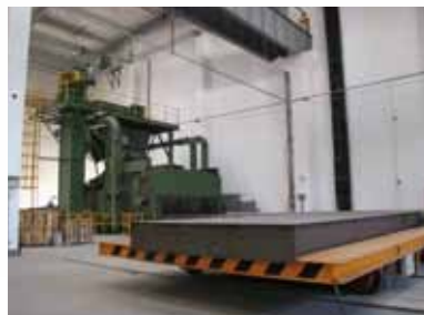
The steel in the VTC205 is shot blasted to create a fantastic painting surface
