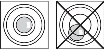
The weigh unit is equipped with a level control (level bubble). The weigh unit is completely horizontal when the bubble is precisely in the middle of the level window (left image = properly level, right image = not properly level).
