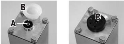
Remove the **white plastic cover** (B) from the weighing cell. This cover protects the **weighing pan support** (A) from damage during transport and keeps liquid from penetrating into the weighing cell during cleaning. Therefore keep the cover in a safe place!
