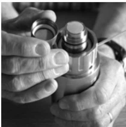
Fig. 3: Sensor with removed MembraCap
