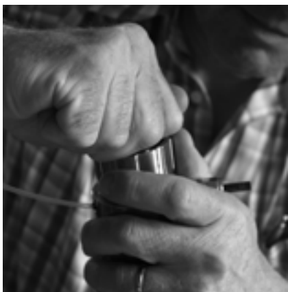
Fig 6: Screwing on the new MembraCap
