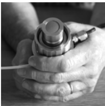
Fig 7: Sensor with newly mounted Membracap, ready for calibration
