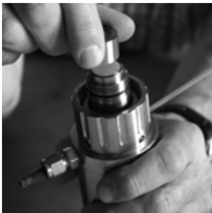
Fig 5: Placing the new MembraCap on top of the Sensor
