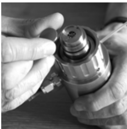
Fig.2: Sensor view with removed Diffusor
