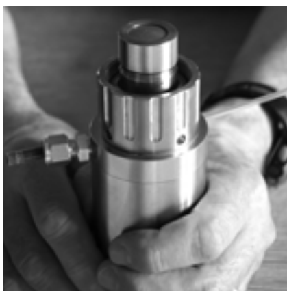
Fig.1: Hold Sensor in upside down position during maintenance eg Membarcap Change
