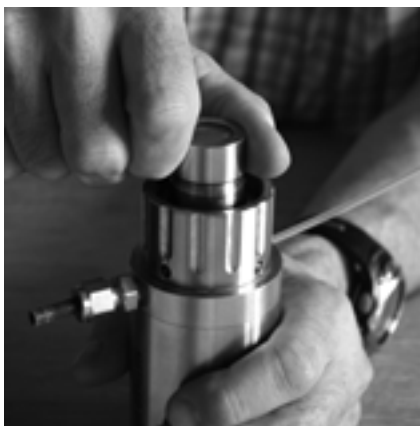
Fig 4: Unscrewing Membracap counter clock wise
