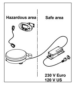
Install the power supply in the safe area near a wall socket.
