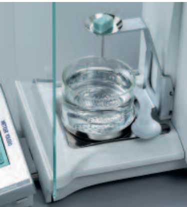
With a keystroke you start the determination. Now you prepare the sample for weighing in air.
