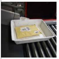
Measure smaller items transported in totes. Dimensioning technology separates the tray from the package.
