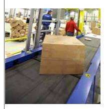
Combine dimensions with weight to establish an object's billable weight. Data is automatically transferred to the host and invoices updated.
