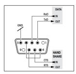
Every balance is equipped with an optional RS232C interface for connection to a peripheral device (e.g. printer, auxiliary display or PC with a 9-pin male connector, see Section 6.4). The balance must then configured to suit the peripheral device in a menu dialog (Sections 4.3.9 - 4.3.12).
