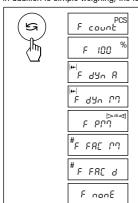
F count Piece counting F 100 % Percent weighing F dYn A Dynamic weighing with automatic start F dYn M Dynamic weighing with manual start
