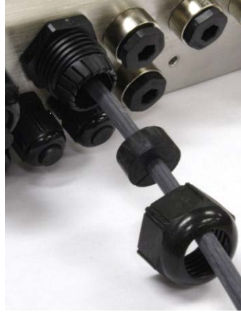
Figure A-23: Cable Inserted Through Grommet, Nut, and Cable Grip
