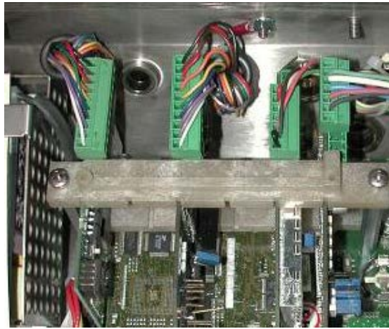
Figure A-20: Shield Wire Termination, Harsh Enclosure
