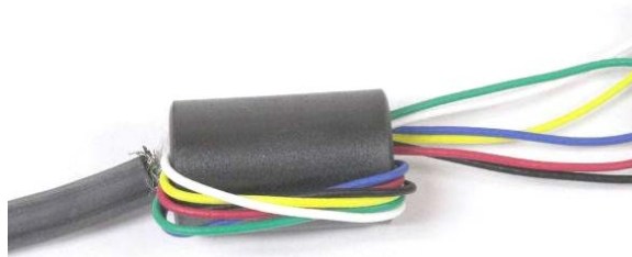
Figure A-16: Ferrite Core on Analog Load Cell Cable
