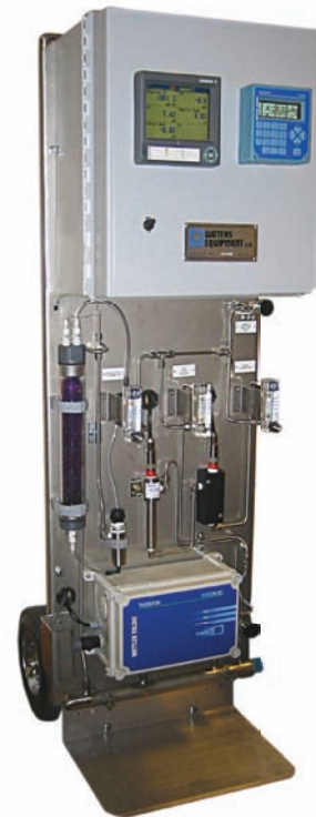
Figure 10 - Portable Verification System including cation Conductivity, pH, DO and TOC Measurements and Data Acquisition (courtesy Waters Equipment)
